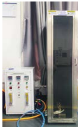
单根垂直 燃烧试验机 Vertical Burning Testing Machine For Single Wire And Cable
